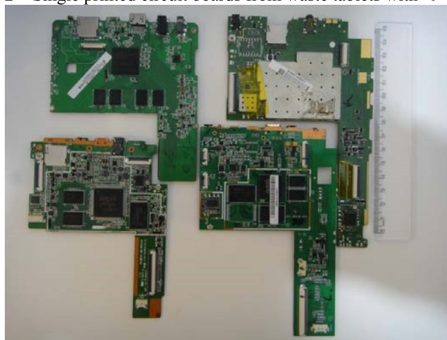
Figure 2 – Single printed circuit boards from waste tablets with “9” format.
