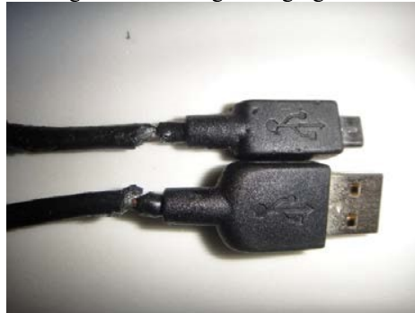
Figure 4 – Damage charging cable
