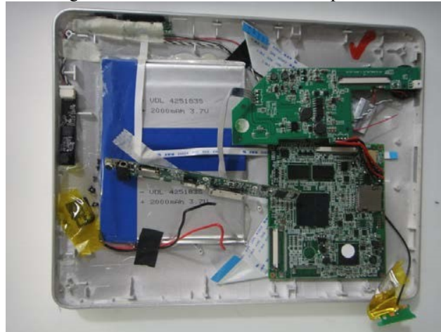
Figure 3 - Oldest tablet model with split PCB.
